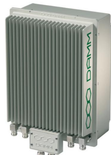
The BS421 is optimised to work together with the DAMM SB421 Service Box, which contains the base station controller software, a AC rectifier providing -48V DC for up to two BS421 base stations. Please request the product sheet for SB421.
